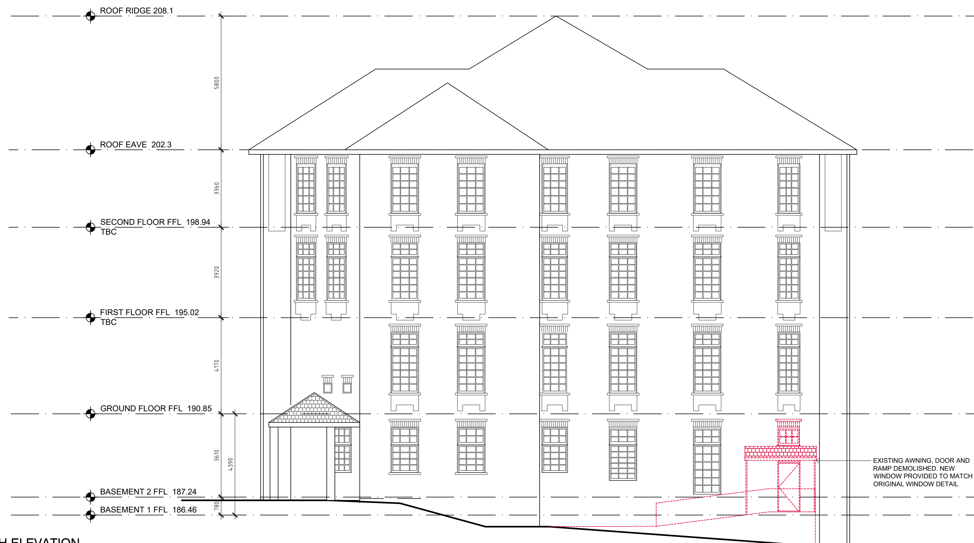
2 EXISTING SOUTH ELEVATION 1101 1:100
